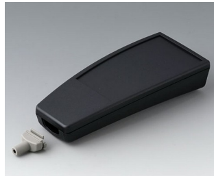
A9068129 SMART-CASE XL, Vers. III ABS (UL 94 HB) black RAL 9005 168x74.4x35.4mm IP 65 opt., IP 40
